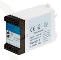
During filling or decanting processes involving solid or liquid materials in the Ex area, the Terracompact IITCO030 automatically identifies faulty or defective ground links in the installation. If the floating changeover contact is switched accordingly, it shuts off the process.
