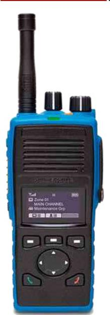
Professional range of ATEX IIA & IIC certified radios. The rugged DTEx Series delivers exceptionally loud audio coupled with outstanding audio clarity, plus the ergonomic controls are specifically designed for gloved hand use.
